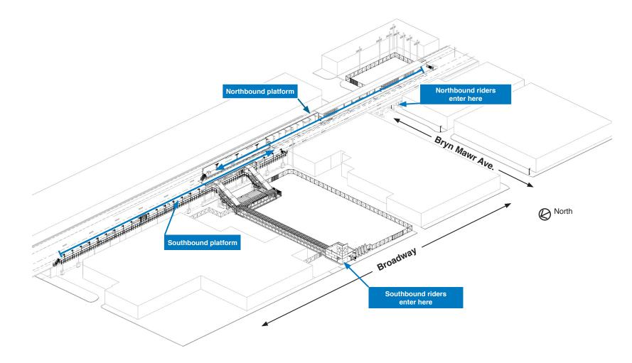
Stage B will require shutting down the existing southbound Red and Purple Line tracks and moving all trains onto the new northbound track structure built in Stage A.
