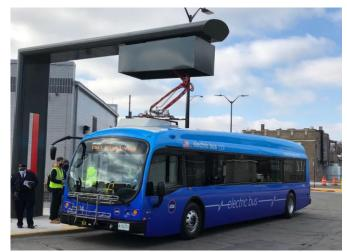
A new CTA electric bus uses the high-powered overhead charger at the Chicago Ave / Austin Blvd bus-turnaround
