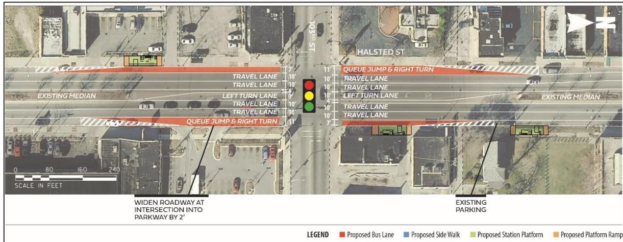
As noted in Table 3.1, the addition of queue jumps would save an average of 4 to 8 seconds per intersection, which would improve bus travel time and reliability at each of the signalized intersections along the South Halsted Corridor. Overall impacts to traffic are anticipated to be low, with some minor impacts to general traffic at intersections.
