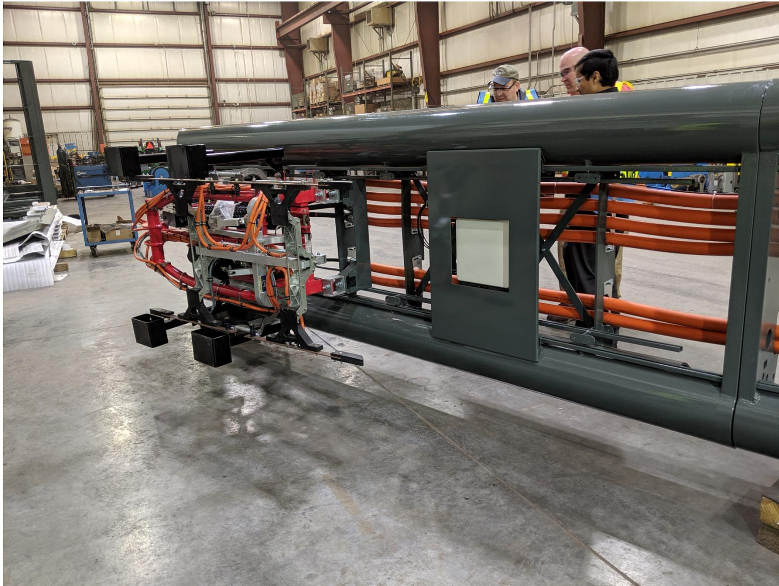
**The Pantograph – Part that connects with the top of the bus**
