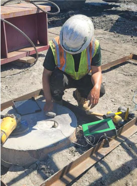
**Pile Integrity Testing**
