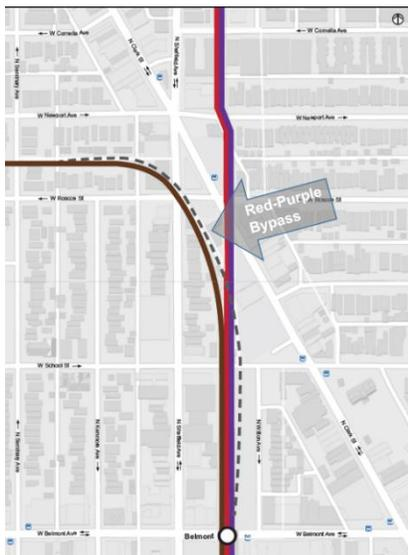
The new Red-Purple Bypass is an important part of CTA's work to improve Red Line service throughout the region. The bypass eliminates a 114-year-old rail junction that had become a chokepoint for service across the CTA rail system and will allow CTA to add rail service during busy travel periods and reduce overcrowding and delays.
