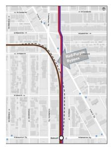
The new Red-Purple Bypass is an important part of CTA's work to improve Red Line service throughout the region. The bypass eliminates a 114-year-old rail junction that had become a chokepoint for service across the CTA rail system and will allow CTA to add rail service during busy travel periods and reduce overcrowding and delays.
