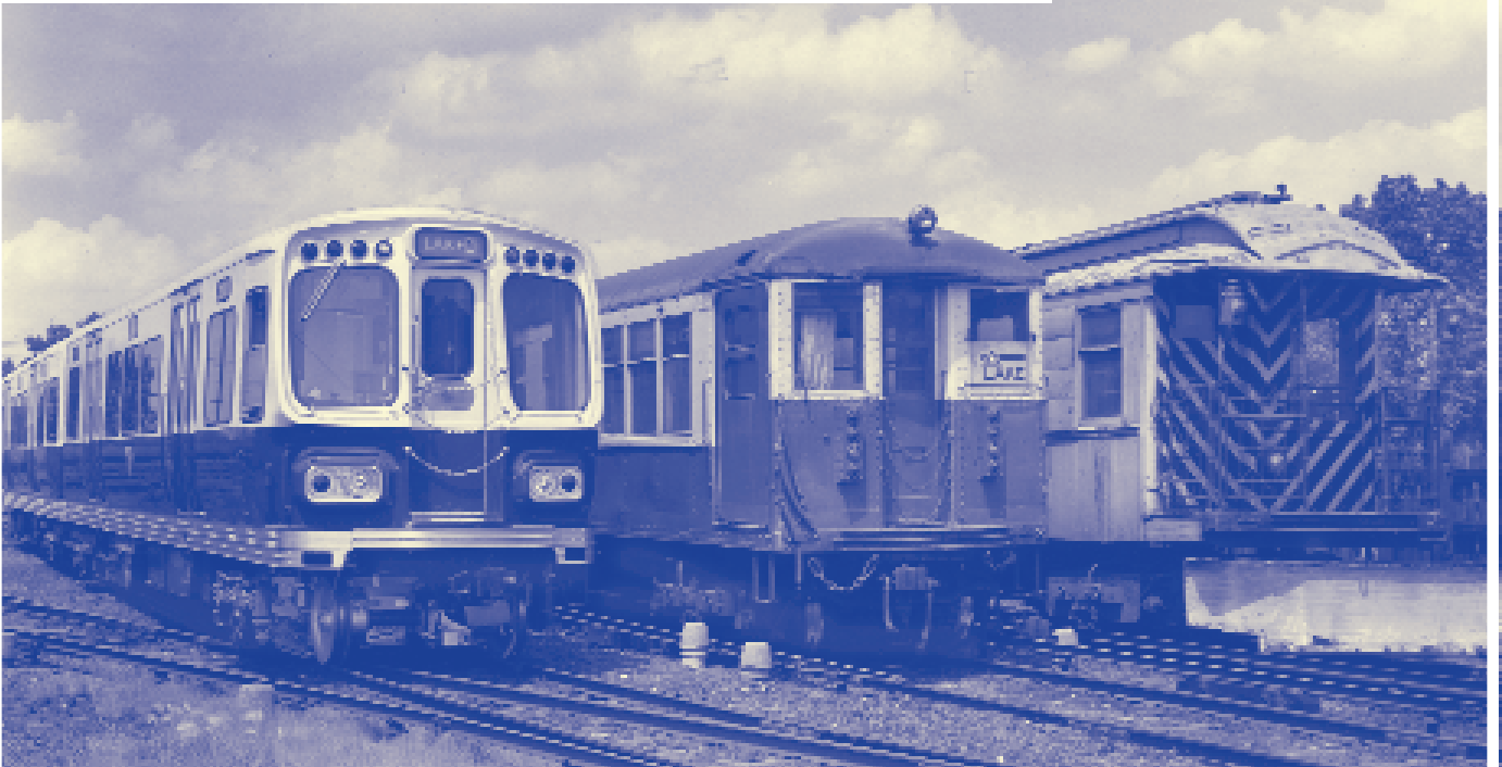
This view at CTA's Hamlin Yard in 1964 shows three distinct types of equipment that had operated on the Lake Street 'L' (now the Harlem branch of the Green Line) from the beginning of its operation. At left, air-conditioned car 2011, built by Pullman, represented the state of the art rail car of the time. Car 4145, center, represented the steel cars that had served the line since 1924. At right, car 3146, by then in work service, had served the route from 1893 to 1954.
