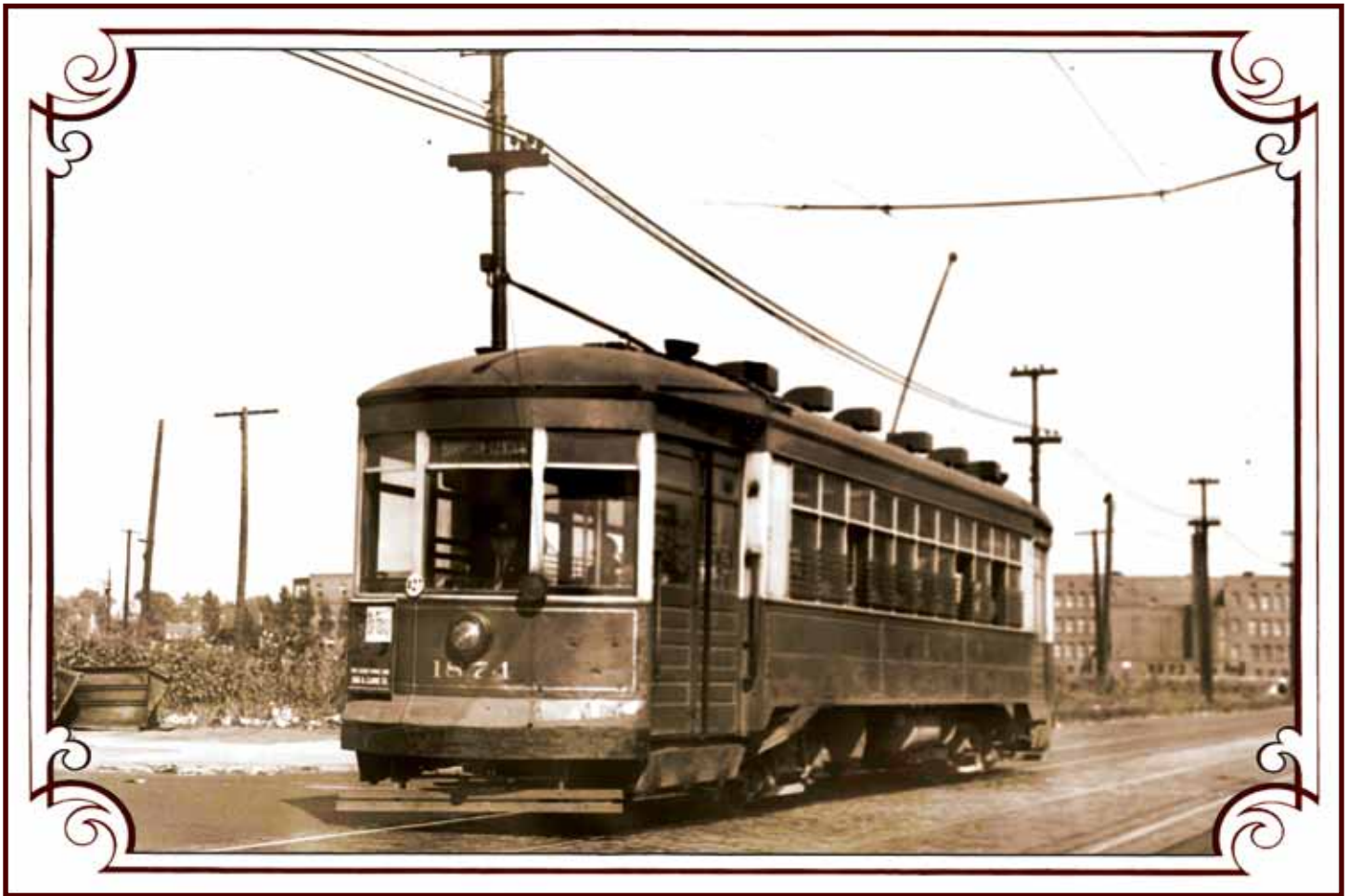
Chicago Surface Lines streetcar 1874, traveling west on Harrison at Laramie near the end of the line at Central, was originally built in 1913 in the Chicago Railway' shops for their own street railway.
