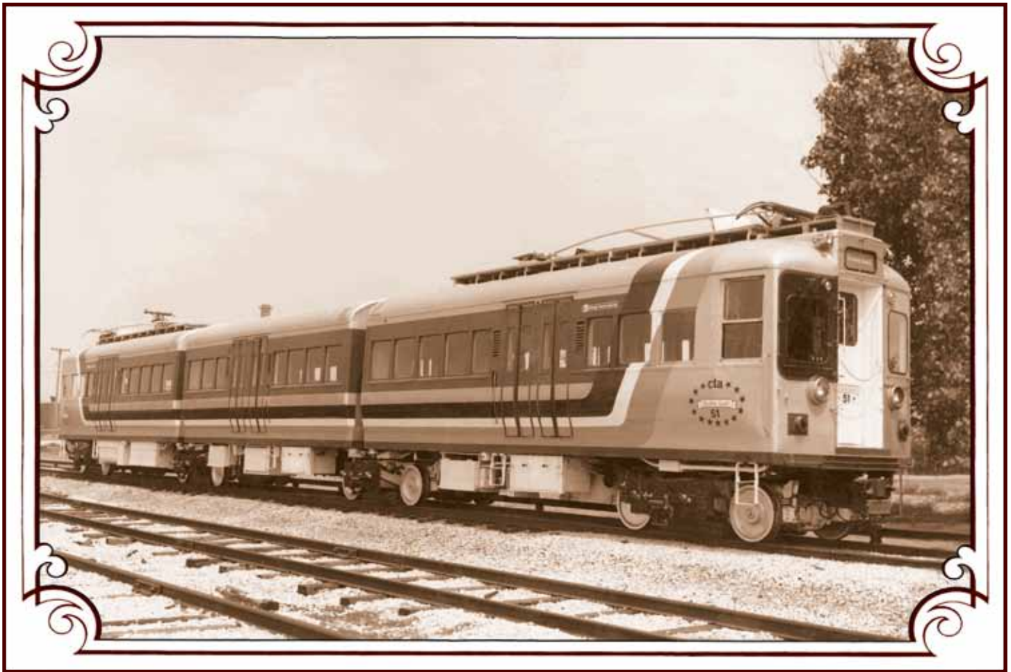
CTA articulated car 51 is seen here at Skokie Shops yard in its sparkling paint scheme commemorating the United States Bicentennial. Four prototype three-section articulated train sets were delivered to the CTA and its predecessor company in 1947-48. These cars, on which the later 6000-series cars were based, were used until 1985.
