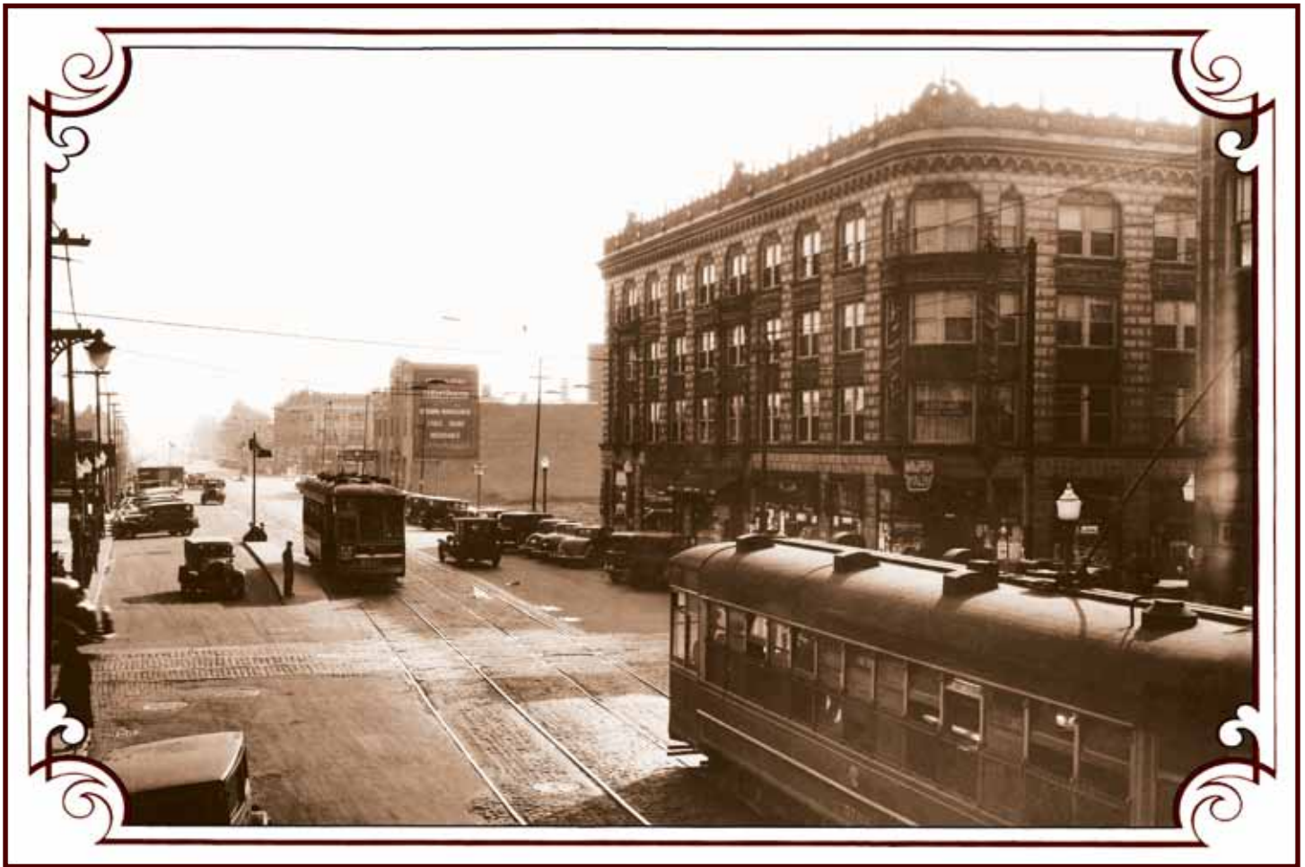
Chicago Surface Lines streetcars 5731 and 5763 are seen on Cottage Grove converging on 79th Street from opposite directions, in this March 1934 photo. These cars were part of a fleet built by J. G. Brill in 1908, and were nick named "Nearsides," or "Muzzleloaders," since both entrance and exit were at the front.
