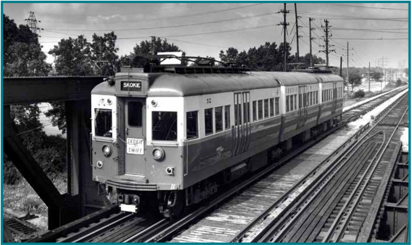
CTA articulated car #52 is seen crossing the bridge over McCormick Boulevard and the North Shore Channel as it operates on the Skokie Swift line, known today as the Yellow Line. This series of cars were three-section articulated units, rather than separate cars. They operated on various parts of the system, somewhat as orphans as no additional cars of this configuration were ordered, but found a suitable home when they were assigned to the Skokie Swift line after its opening in 1964.
