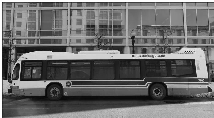
Earlier this year, CTA received the first of the 300 new 40-foot “standard” size clean diesel buses manufactured by Nova Bus. The new buses, which replace those purchased in 2000-2002, are more fuel efficient, have brighter LED lighting and are equipped with 10 surveillance cameras.
