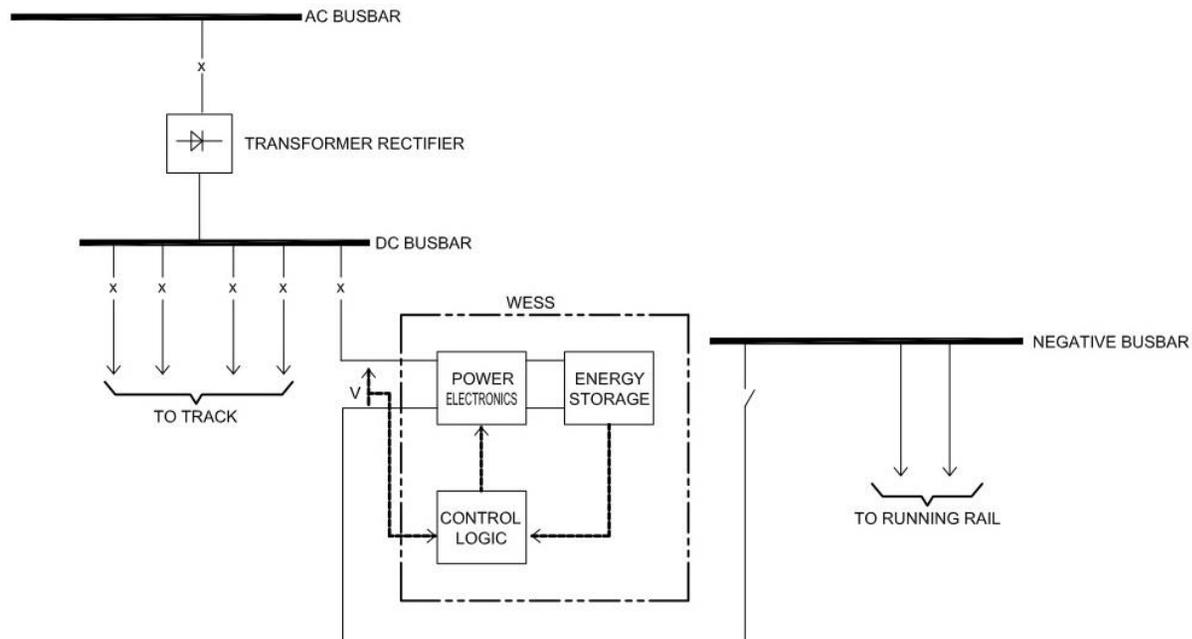
Figure 4-1: Single Line Diagram of a WESS
