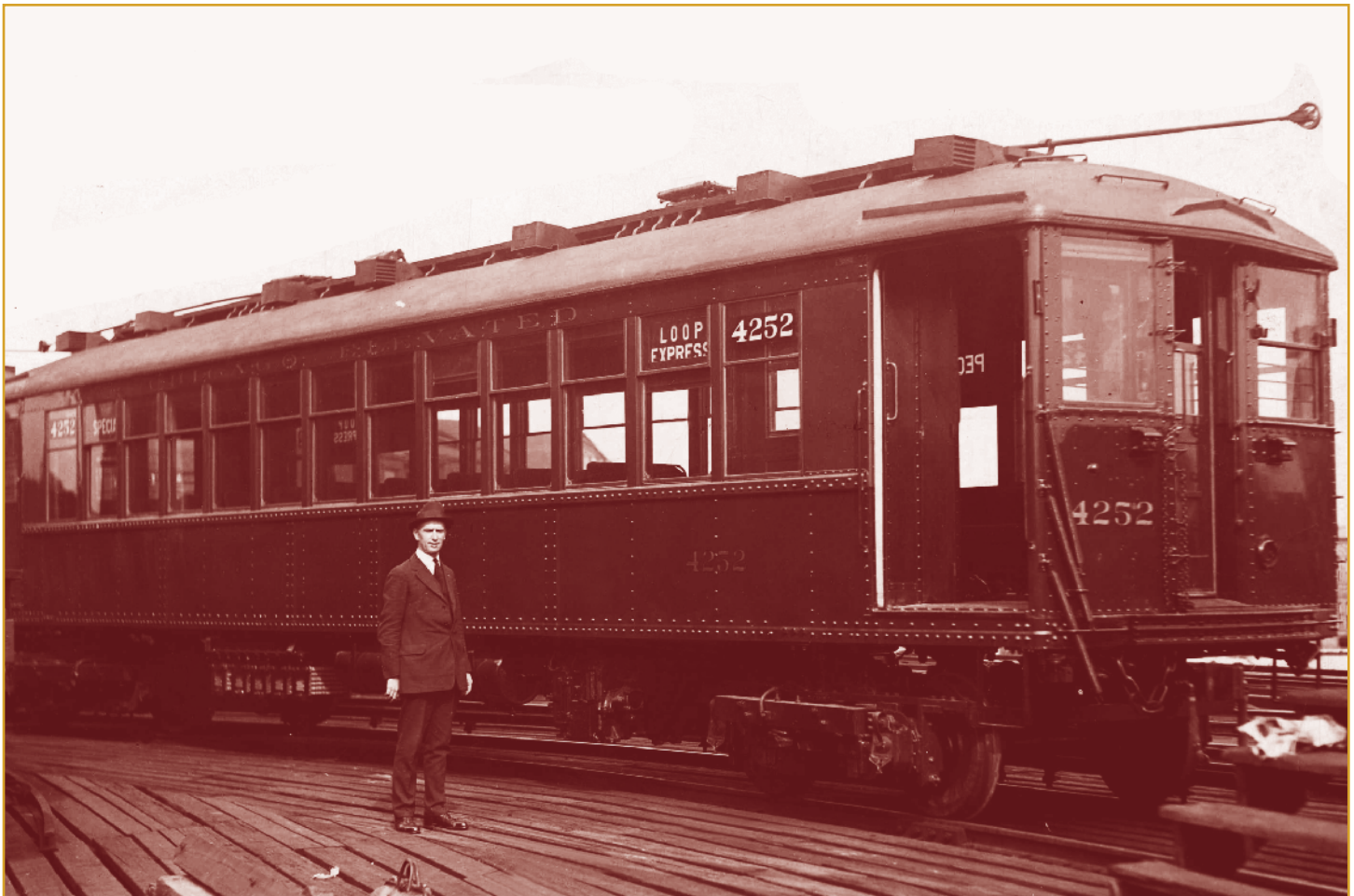
It is 1923 and Chicago Elevated Railway car #4252 has just been received from its builder, Cincinnati Car Company. The 4251-4455 group of 4000-series cars featured the newest amenities of the time, including plush seats and electric fans for the passengers' comfort, and new shaded lighting.
