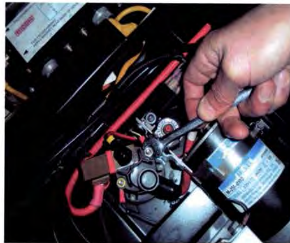
Step 27. Using a 3/8" wrench, install and tighten the nuts on the terminals
