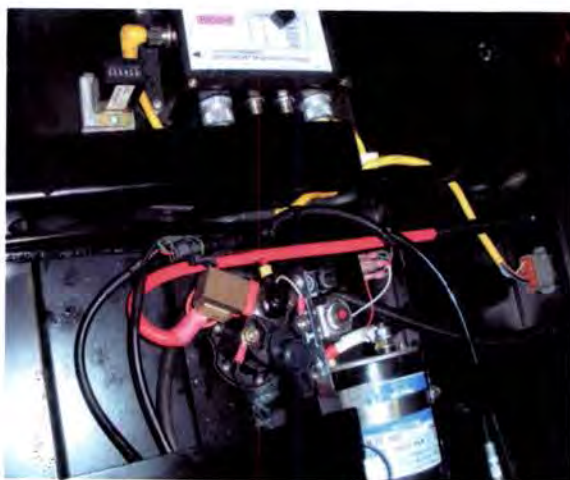
Step 28. New solenoid installed
