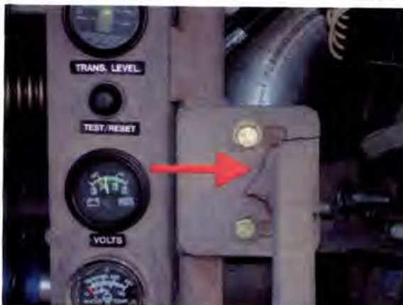
FIGURE 7: SHOWING TYPICAL CRACKS ON BELT GUARD STRUTS.
