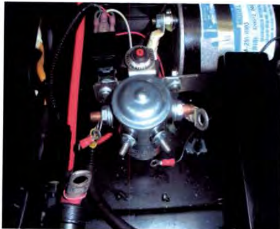
Step 8. Solenoid with all connections removed
