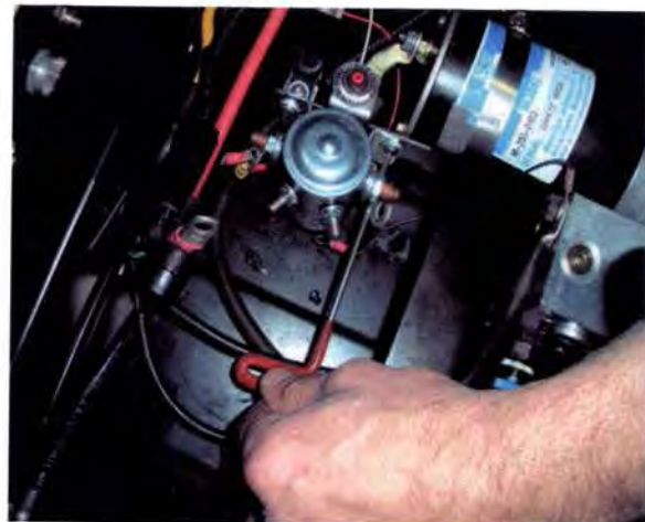
Step 9. Loosen the right side mounting screw and completely remove the left side mounting screw
