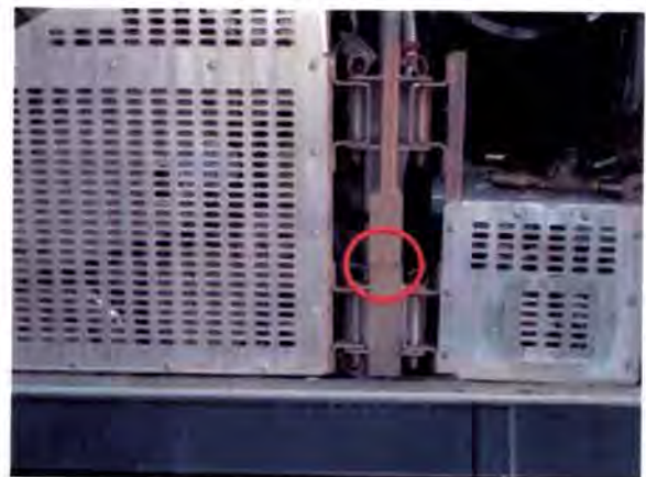
FIGURE 7: SHOWING TYPICAL CRACKS ON BELT GUARD STRUTS.
