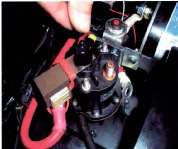
Step 21. Install and tighten the 1/2" nut and install the dust boot over the exposed stud
