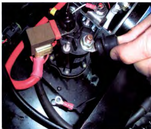
Step 24. Install and tighten the 1/2" nut on the solenoid
