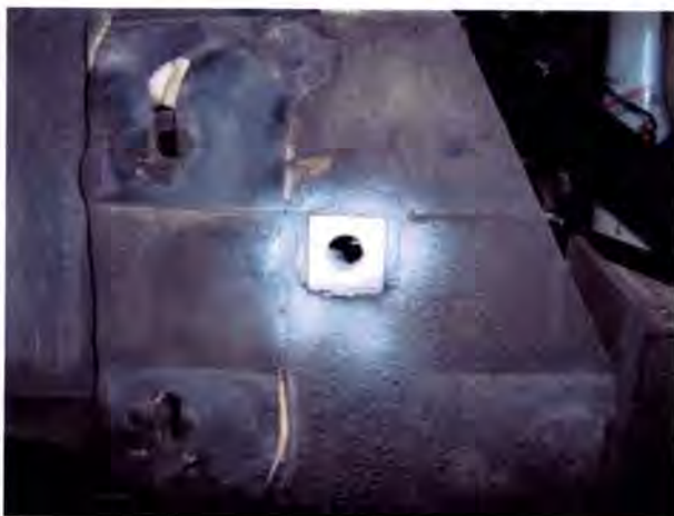
FIGURE 3: SHOWN VIEWS OF THE MATING SURFACE TO BE CLEAN (WITH NO CORASHIELD) TO APPLY ENGINE STRUTS/HARDWARE TO ACHIEVE PROPER HARDWARE TORQUE. CHECK MATING SURFACE AT THE FORWARD LOWER MOUNT.
