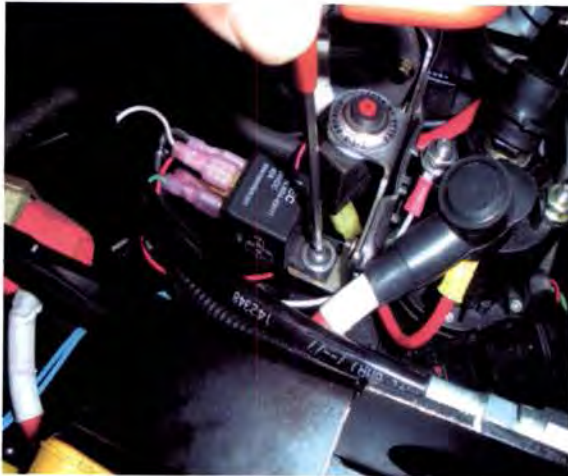
Step 29. Removing "old" relay mounting screw
