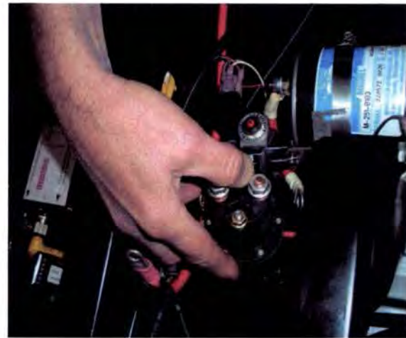
Step 11. Install the new solenoid by inserting the right mounting tab into the right mounting screw
