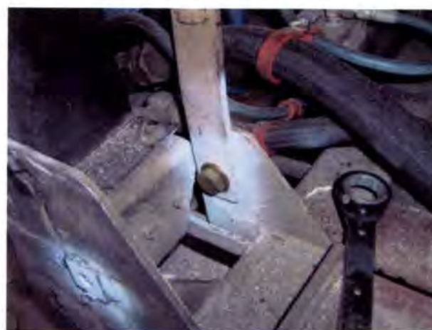
FIGURE 3: SHOWN VIEWS OF THE MATING SURFACE TO BE CLEAN (WITH NO CORASHIELD) TO APPLY ENGINE STRUTS/HARDWARE TO ACHIEVE PROPER HARDWARE TORQUE. CHECK MATING SURFACE AT THE FORWARD LOWER MOUNT.
