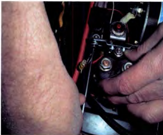
Step 12. Install left side mounting screw and tighten both sides
