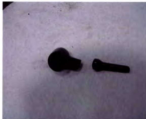
Step 13. Cut the provided dust boot as shown above
