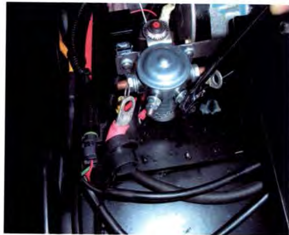
Step 7. Using a 3/8" wrench, disconnect the black and white terminals from the solenoid
