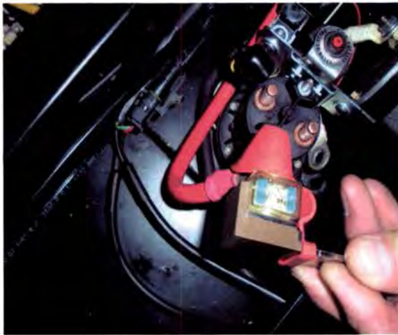
Step 18. Cover the fuse block stud with it's supplied protective boot
