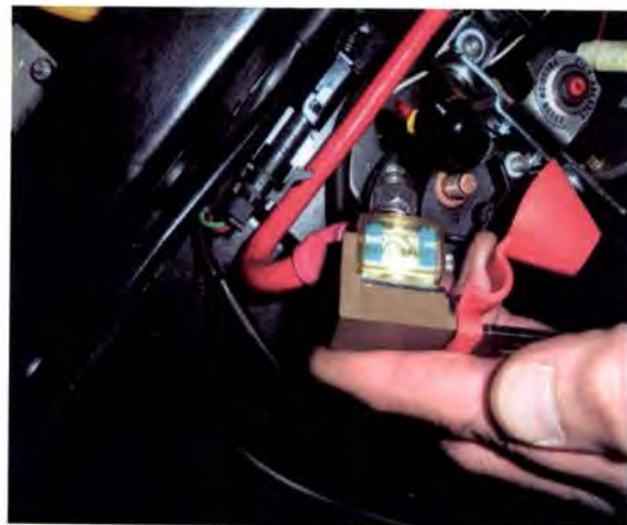
Step 17. Tighten the fuse block to the main power cable using a 1/2" wrench
