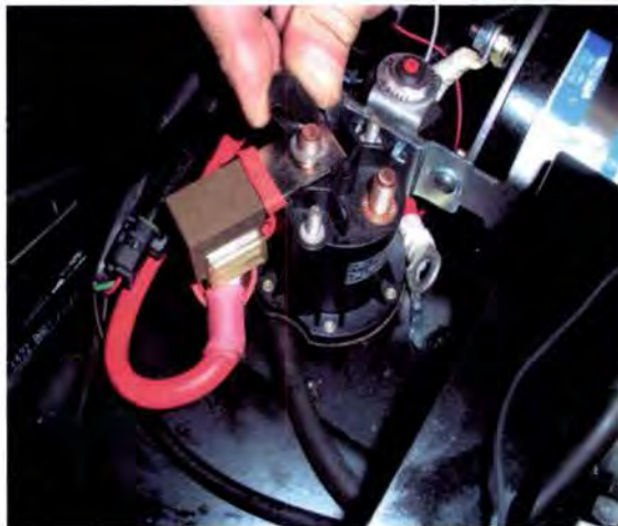
Step 20. Install the circuit breaker power cable to the solenoid
