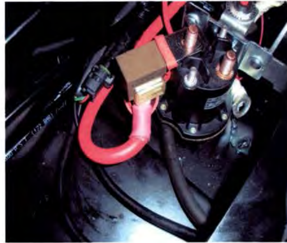
Step 19. Install the fuse block onto the solenoid
