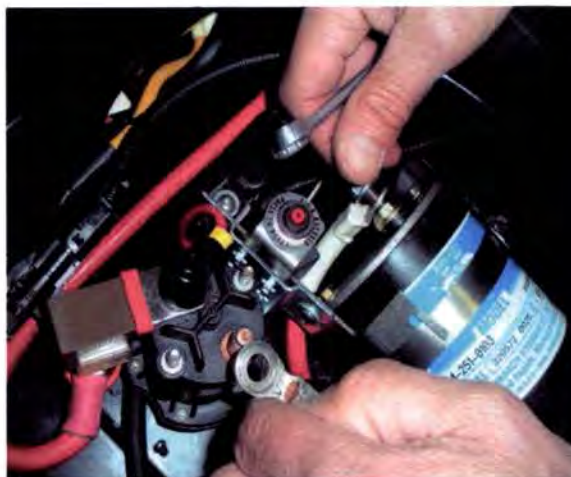
Step 23. Install the other end of the motor power cable onto the solenoid
