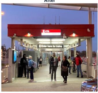
47th Red Line – New LED wall pack lightening installed, and back lightening added to signage for better station visibility
