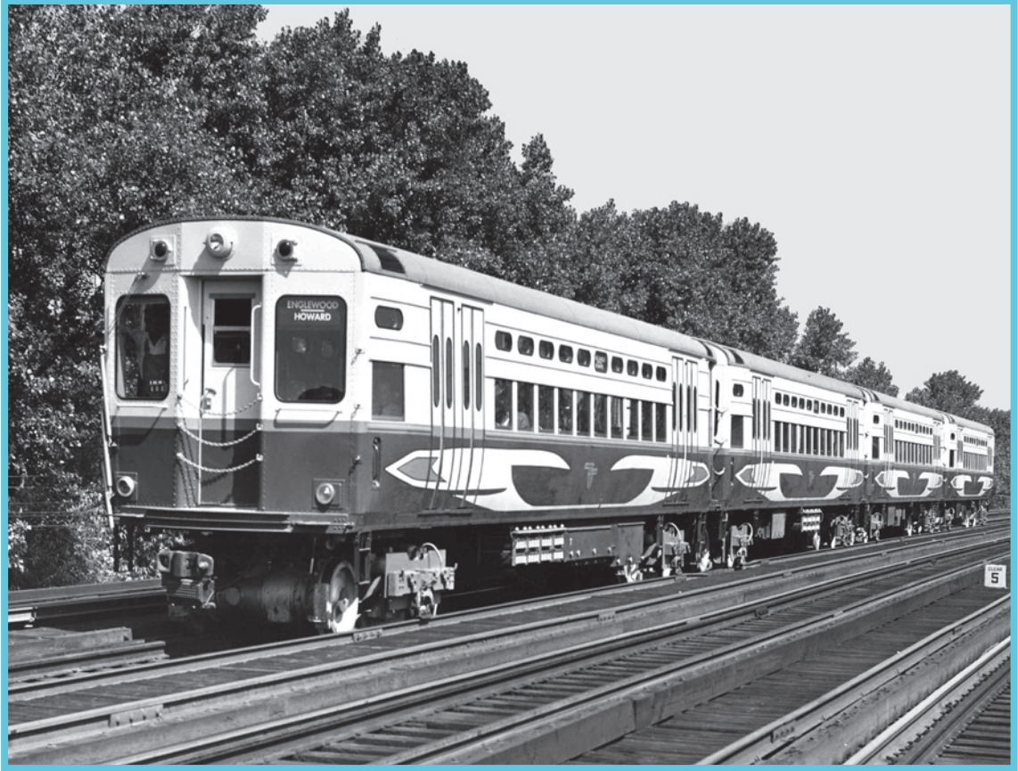
A four-car train set of 1-50 series cars, consisting of cars 1 through 4, is seen here in 1960 in a special livery of maroon, red, cream and silver with a distinctive stylized arrow design to differentiate them from the rest of the fleet on the system. Built by the St. Louis Car Company, cars 1-4 were designed to test new "high performance" equipment for improved acceleration and speed.
