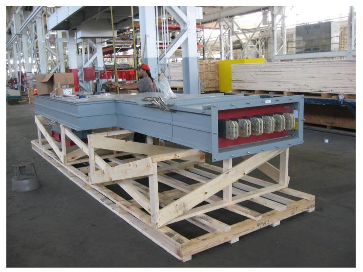
**Bus Duct Assembly for Princeton Substation at Factory**
