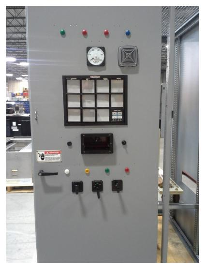
**Rectifier Control Cabinet for Princeton Substation in Factory**
