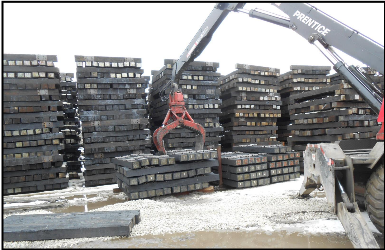
Storage of pre-plated ties
