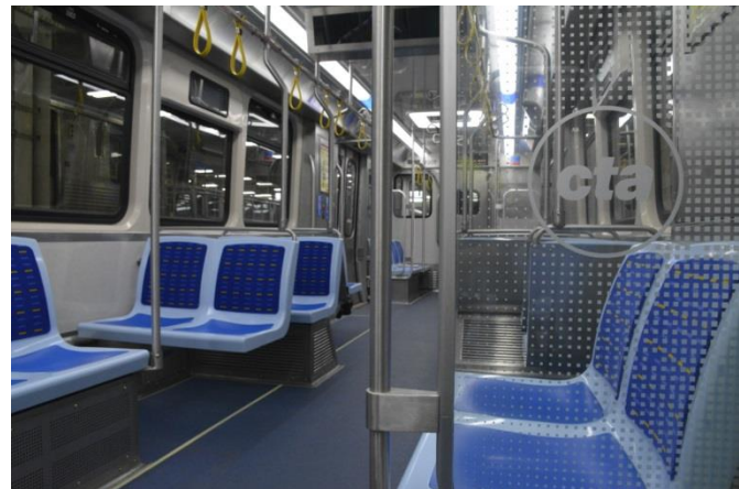
Top photo: Exterior of new 7000-Series rail cars. Bottom photo: Interior of new 7000-Series rail cars, which will have a variety of new features including center-aisle grab bars, clear windbreak panels, added LED information displays and a refreshed seating configuration.
