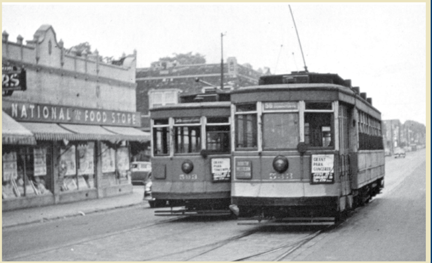
Two Pullman-built “Red Rockets” – cars 593 and 533 – pass each other on Milwaukee Avenue in the early 1950’s. Also known as “Big Pullmans,” these cars could accommodate great numbers of passengers, making them ideal for use on high demand routes in the city. Red streetcars last operated May 30, 1954, and all streetcar service in Chicago ended June 21, 1958.
