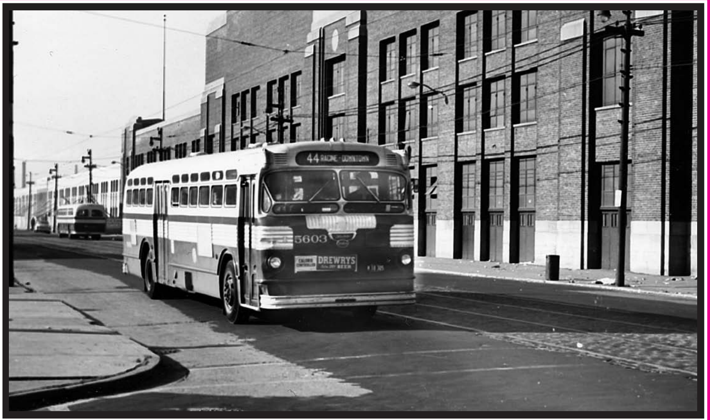
A 5500-series propane bus (circa 1950) built by Flixible is shown operating on the #44 Racine route from 87th/Racine to the Loop. Bus #5603 is pictured in front of Chicago's International Amphitheater which stood at Halsted and 42nd streets until it was demolished in 1999.
