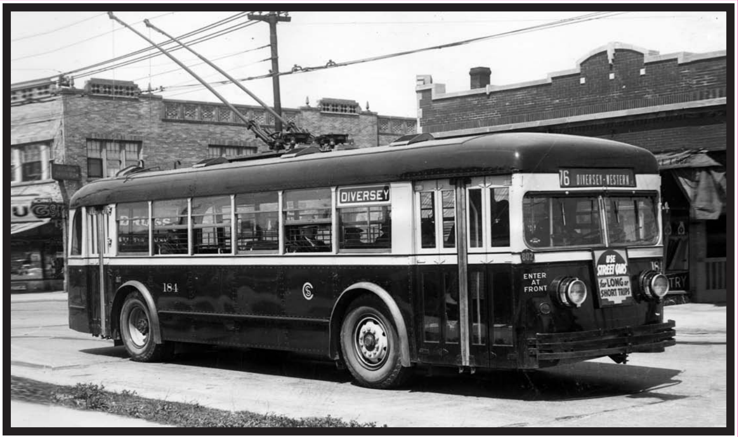
Chicago Surface Lines (CSL) trolley bus #184 was brand new when this photograph was taken in 1936. This was one of 15 buses built by the St. Louis Car Company for use on the CSL's small northside trolley bus network.
