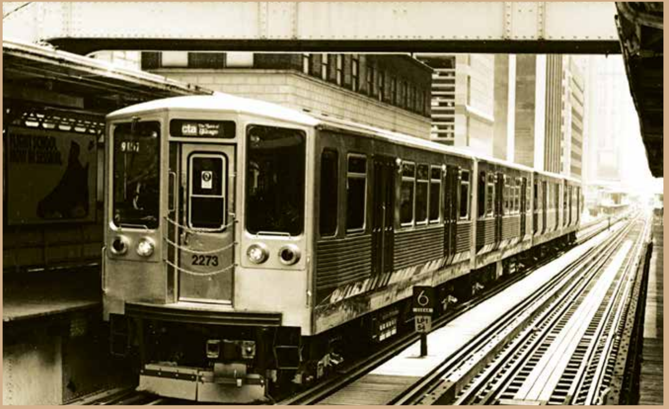
A four-car train of 2200-series cars, headed by car #2273, is berthed at the former Randolph/Wells station on the Loop Elevated. Purchased by the City of Chicago as part of a grant that also funded the construction of the Dan Ryan and Kennedy extensions, their design was intentionally boxy and rectilinear to harmonize with the International architectural style utilized by designers Skidmore Owings and Merrill for the Kennedy and Dan Ryan (KDR) stations.
